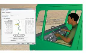
With Jack and the OPT, you can interactively evaluate a concept vehicle design for human fit and performance. Since Jack is infinitely scalable, you can create a male or female figure of any desired size, and the OPT functionality will automatically position the figure into the vehicle based on validated research models. You can further investigate your design by using the comfort analysis and vision analysis functionality to improve occupant
