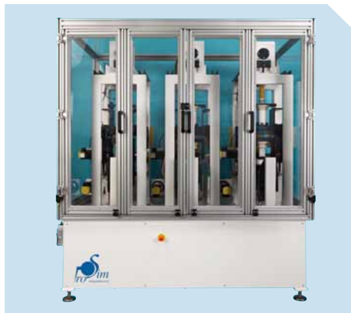
A three-station independently controlled knee wear simulator with a close-up of a soak station
