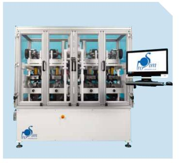
Six-station hip and spine simulator with close-up view of the dual soak-stations
