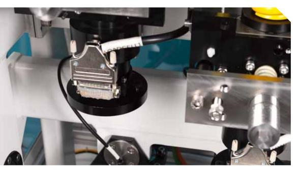
Six-axis load cells provide monitoring of all forces and torques applied to the cup or upper vertebral body in the six-station hip and spine simulator
